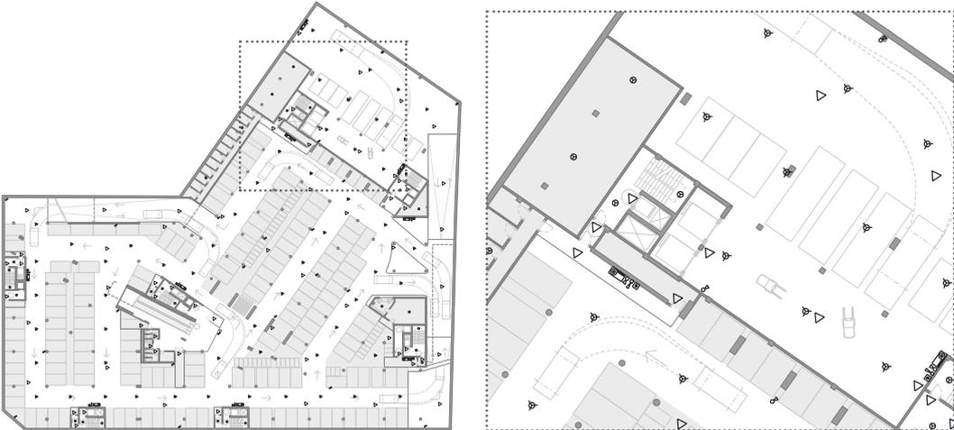
The top section shows a floor plan on the left and a detailed view on the right. The floor plan has a dashed black box around a specific area. The detailed view shows a staircase and surrounding rooms with black icons for fire extinguishers and emergency lighting. The fire extinguishers are represented by a square with a fire extinguisher symbol, and the emergency lighting is represented by a triangle with a light symbol.
