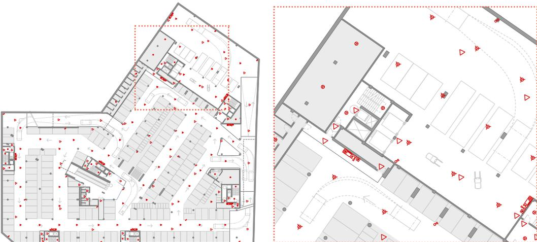
The bottom section shows a floor plan on the left and a detailed view on the right. The floor plan has a dashed red box around a specific area. The detailed view shows a staircase and surrounding rooms with red icons for fire extinguishers and emergency lighting. The fire extinguishers are represented by a square with a fire extinguisher symbol, and the emergency lighting is represented by a triangle with a light symbol.
