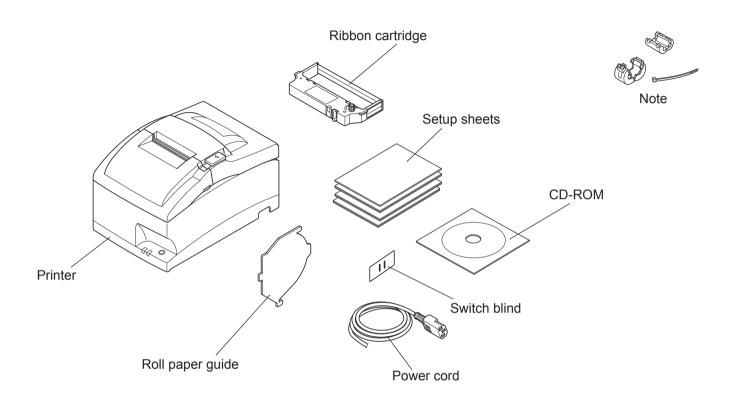
**Note:** The ferrite core and fastener provided with your printer depend on your printer configuration.
