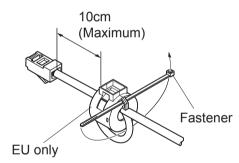
3 Loop the fastener around the cable, and then pull the end of the fastener tightly through its buckle. Use a pair of scissors to cut off the excess end of the fastener.
