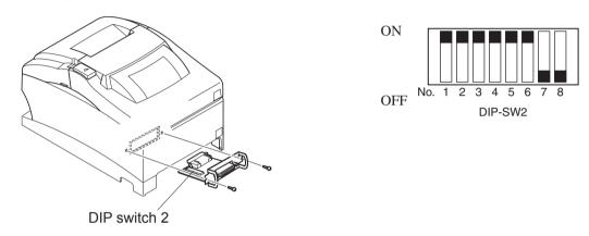
The factory settings of DIP switch are all on, except for switches 7 and 8.
