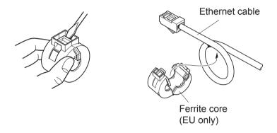
2 Pass the fastener through the holes in the ferrite core as shown in the illustration.
