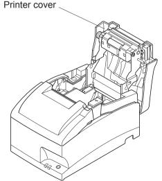
(6) After you have opened the printer cover, remove the four screws to remove the printer cover and reveal the cutter.
