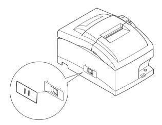
The power switch can be turned ON (|) and OFF (O) by inserting a narrow instrument (ball pen etc) in the holes in the switch blind.
