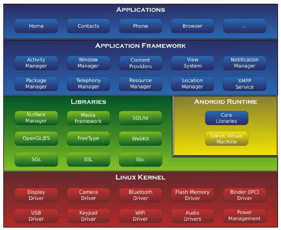
Fig 2-1. Android System Structure
