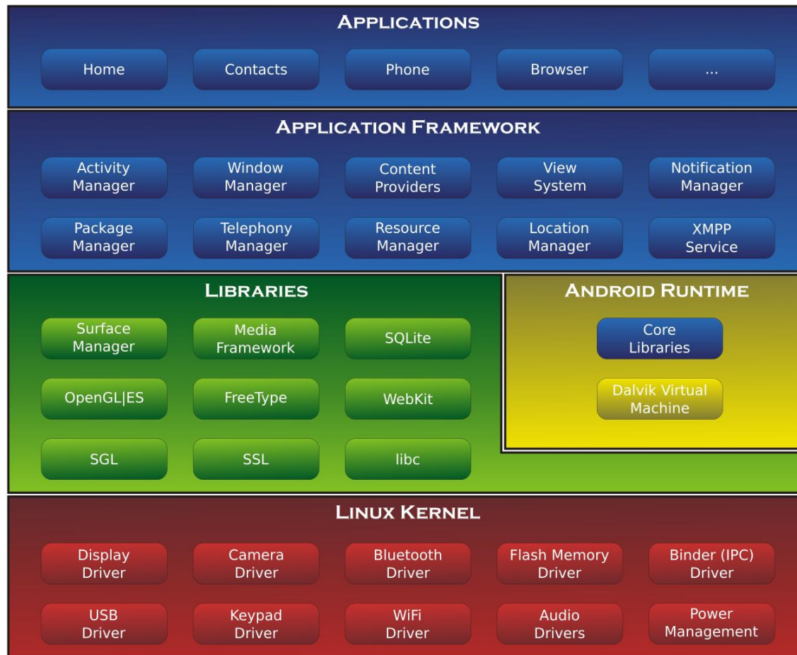
Fig 2-1. Android System Structure
