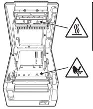
THIS LABEL INDICATES THE RISK OF BURNS DUE TO THE HIGH TEMPERATURE OF THE PRINT HEAD AND A RISK OF BEING CUT BY THE MANUAL AND AUTO CUTTERS WHILE THE PAPER COVER IS OPEN.
