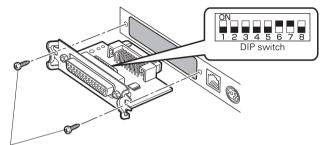
Serial interface board mounting screws
