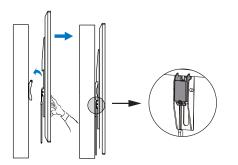
Apply the TV with wall mount to the wall plate
