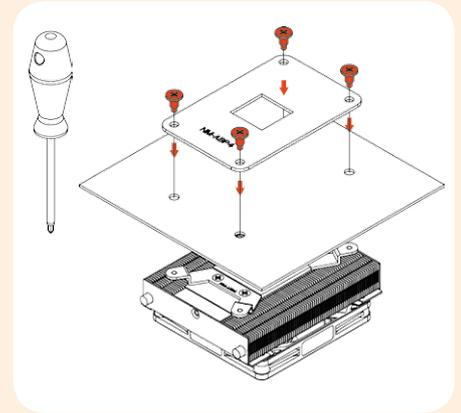
**Caution:** Gently tighten the screws until they stop, but don't use excessive force (max. torque 0.6 Nm).
