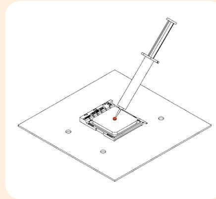
**Caution:** Applying too much thermal paste will lower heat conductivity and cooling performance!
