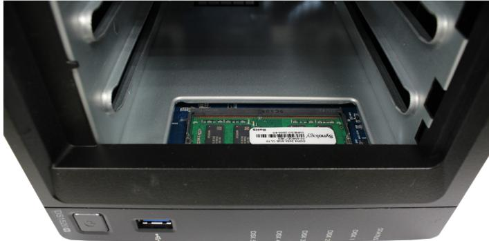
**Note:** When you remove the drive trays, sensitive internal components are exposed. Avoid touching anything other than the memory assembly when removing or adding memory.
