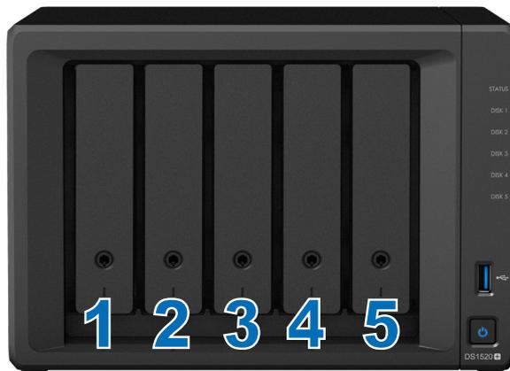
**Note:** If you plan to create a RAID volume, we recommend installing drives of identical size to make the best use of drive capacity.
